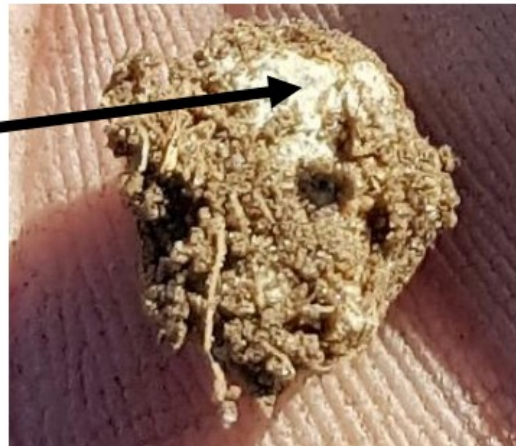
Struvite pellet after 4 months
